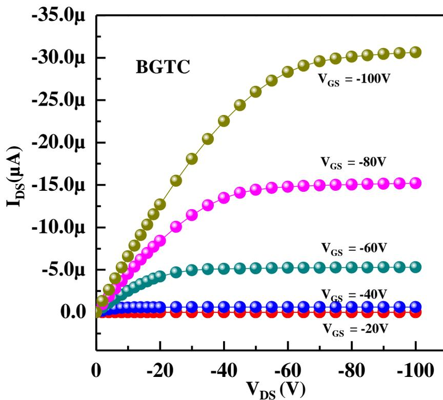
Figure 6.2 Output characteristics of bottom gate top contact structure
