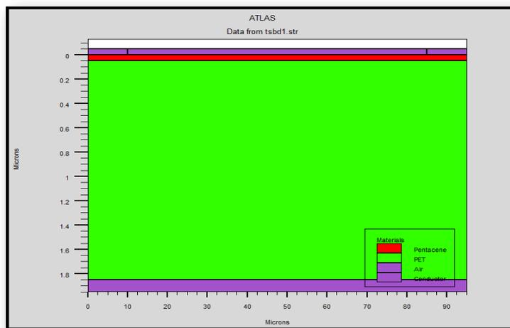
**Figure 5.1 Simulated Structures of (a) BGBC (b) BGTC**
